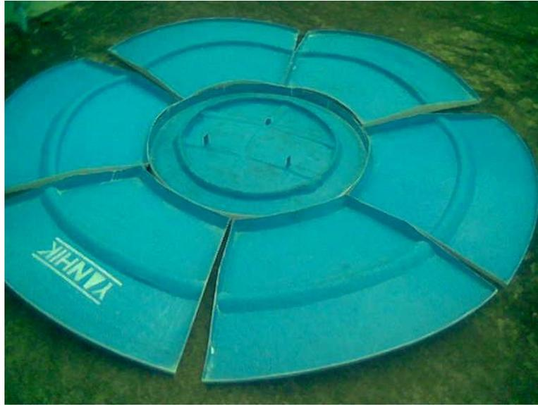
The sun is also brutal on the reflective surface of fiberglass antennas, oxidizing the protective coating and eventually turning the fiberglass to powder.
